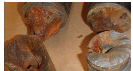
Figure 20: Cracked shaft due to corrosion [Ref: 9.k]
