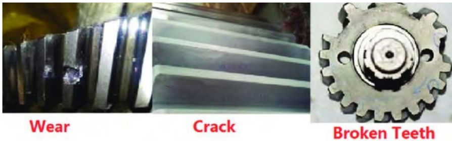
Figure 15: Gear defects [Ref: 9.f]
