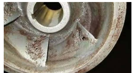
Figure 16: Centrifugal pump blade erosion [Ref: 9.g]
